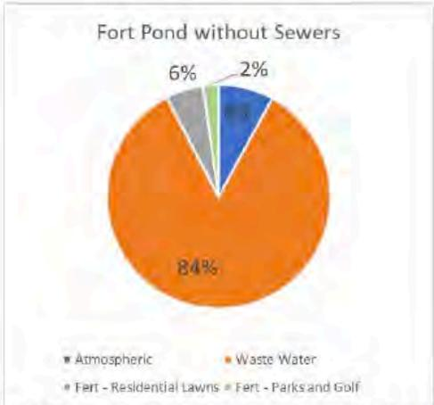
Figure 2 - Components of Nitrogen Budget Prior to Sewers
