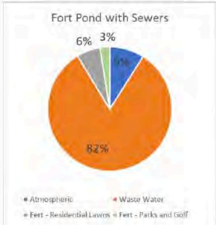
Figure 3 - Components of Nitrogen Budget After Sewers
